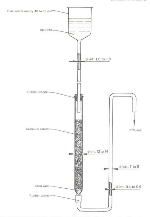
NOTE — A flexible connection may be used between the bottom of the column and the effluent capillary tube, in order to allow adjustment of the height of the capillary tube and thus of the flow rate.
